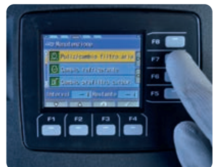
Basic maintenance screen on the 3.5" multi-colour monitor
