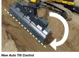
Automatically tilts bucket to design and returns it to horizontal to unload. Makes delivering final grade quicker and easier.
