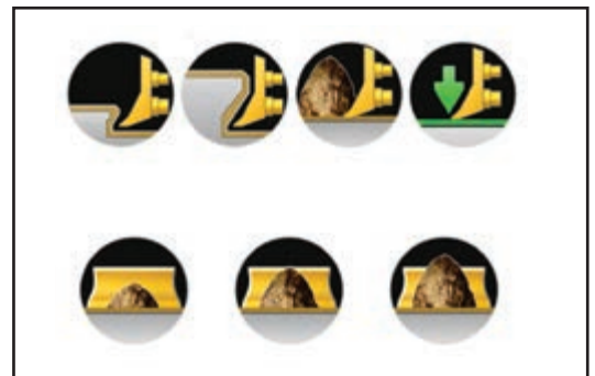
Intuitive selectable load settings – Machine control load settings can be adjusted between presets to tailor response to material conditions.
