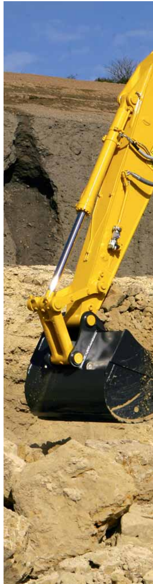
Power mode Boom pushing force is increased, ditch digging and box digging operation on hard ground are improved.
