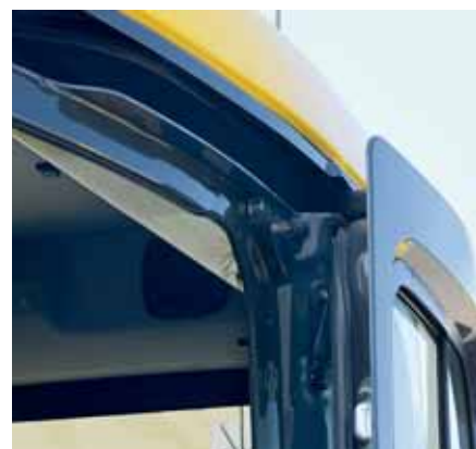
The sliding door facilitates easy entrance in confined areas while reducing the risk of damage on roadways. The cab also features a sliding window.
