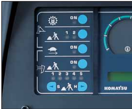
Track shoe slip control panel
